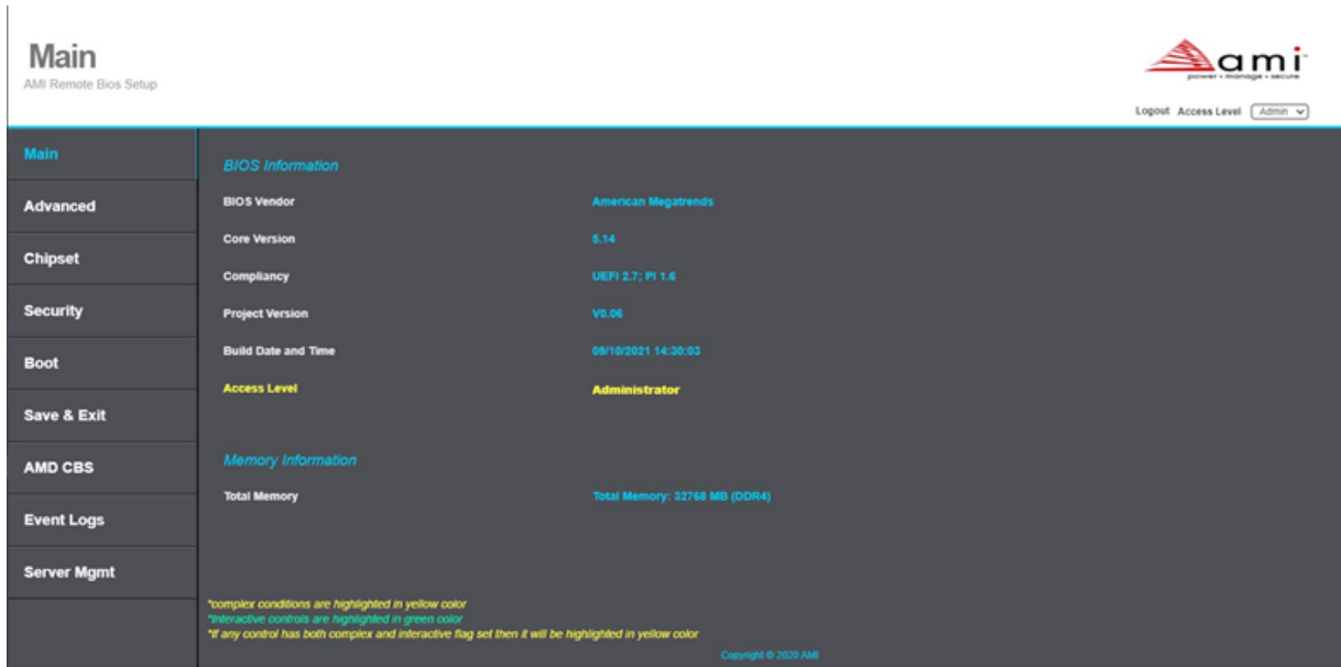
Figure 46 Main menu for ARU version of BIOS setup utility
