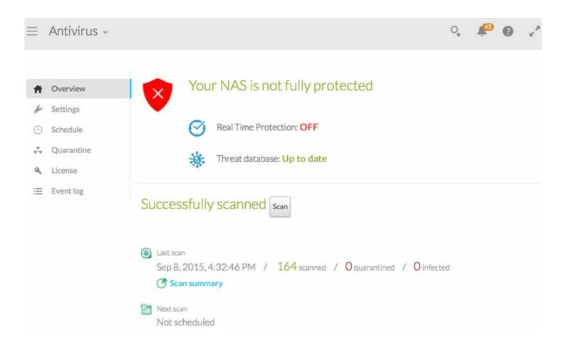
**Important info:** Real time protection is a great option to keep your NAS and its data safe from harmful files. However, enabling real time performance can reduce NAS performance due to the demand upon the CPU.
